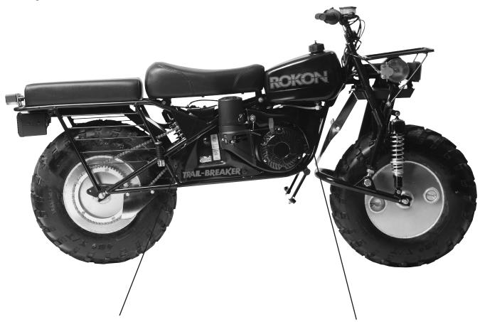
The Vehicle Identification Number is on the center frame tube beneath the driver seat.
