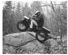
The ROKON is designed with individual disc brakes on the front and rear gear boxes. The front brake (right hand side) will stop both wheels through the gear train. When
