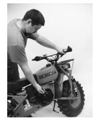
three-range selector in the desired gear range. Put the ball of the foot, rather than the instep on the footrest. Accelerate and ride. Use braking as necessary. Pre-plan your route before attempting to negotiate difficult terrain. Lean into the hill when climbing switch backs. Descend steep slopes at slow speed in low range. Apply rear brake pressure before front brake application.
