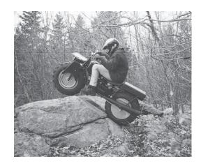
The ROKON is designed with individual disc brakes on the front and rear gear boxes. The right hand front brake will stop both wheels through the gear train. When braking with the front brake, the machine should be in a "straight away" position. Hard braking, with a turned front wheel, can cause loss of steering which can result in loss of control. The left hand rear brake should be used more often for going down steep slopes.
