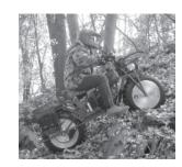
When riding downhill, shift your weight as far to the rear and uphill side as possible. Use low gear and engage the throttle slightly to allow the engine compression to provide braking. Whenever possible ride straight downhill. Turn into corners with the rear brake only, so as not to slide the front wheel and lose steering control.
