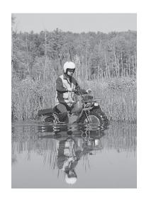
The ROKON can be used to cross slow moving shallow water of up to a maximum of 24 inches in depth. Before entering the water, choose your path carefully. Enter where there is no sharp drop off, and avoid rocks or other obstacles which may be slippery or upset the ROKON. Drive slowly
