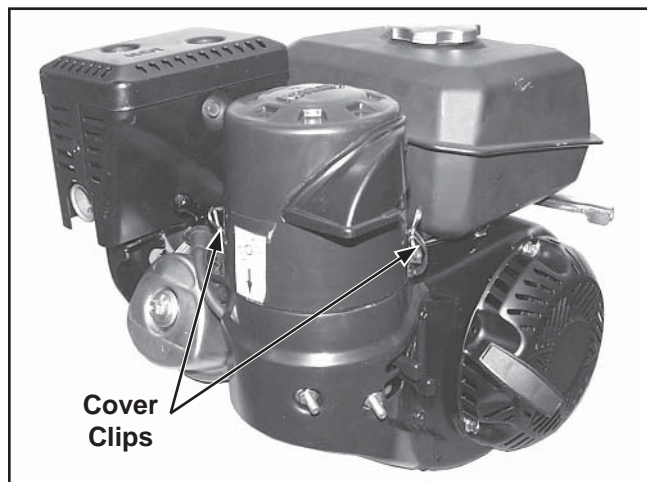
Figure 11-90. Install Air Cleaner Cover.
