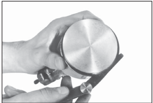
Figure 10-14. Measuring Piston Ring Side Clearance.
